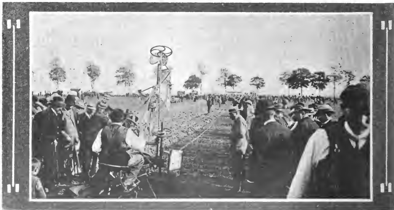
Bajac Plowing Machine at the Arriens Trials—Operated by Winding Drums at Each End of Field
